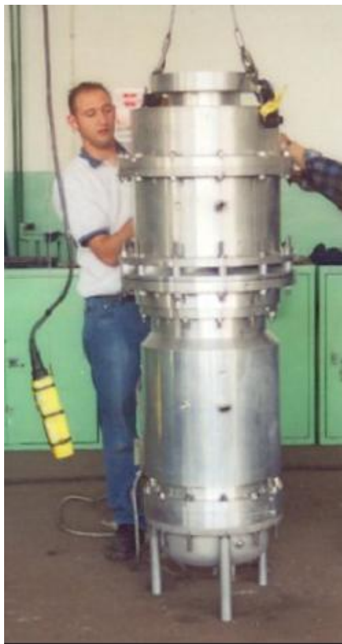
Figure 3. Assembled Two-Phase Expander
