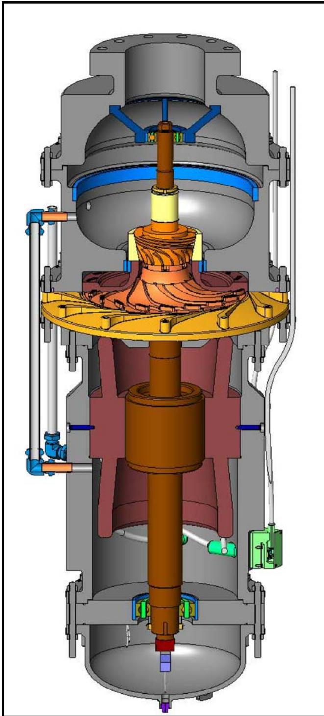
**Figure 4 - Ebara Two-Phase Expander Cross Section.**
