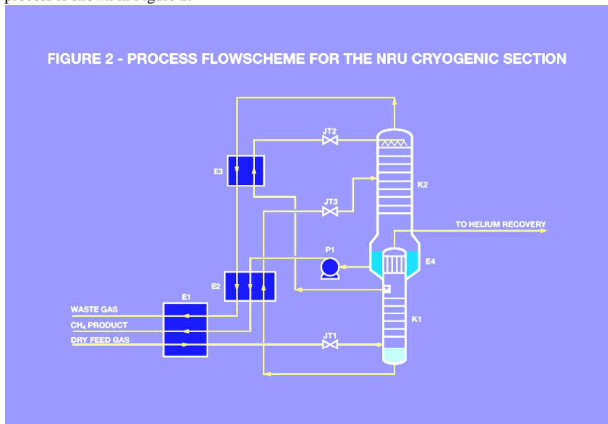
The dry feed gas is admitted into E1 of the cryogenic unit where it is cooled at 5.3MPa, condensed and subcooled before it is passed through JT1 for expansion to the lower column K1. The pressure in the lower column is about 2.1MPa and thus there is some flash into the lower column. The “rich liquid” from the base of K1 is then subcooled in E2 against returning
