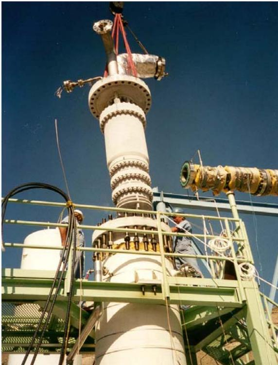
Figure 7: Variable Speed LNG Expander on the Test Stand
