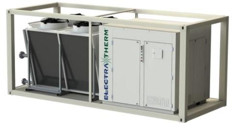
The package is available at the Manufacturer's Suggested Retail Price (MSRP) of €193,000/US\$262,000. Product details are available [here](#). The Green Machine 4011-F generates fuel-free, emission-free electricity utilizing waste heat between 77-116°C (170-240°F) and flow rates between 3.2-12.6 l/s (50-200 GPM) to produce up to 35kWe.
